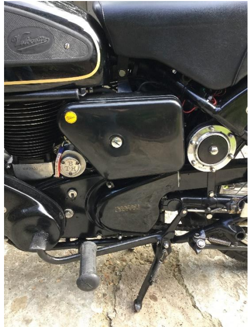
Badge covering original key switch hole
