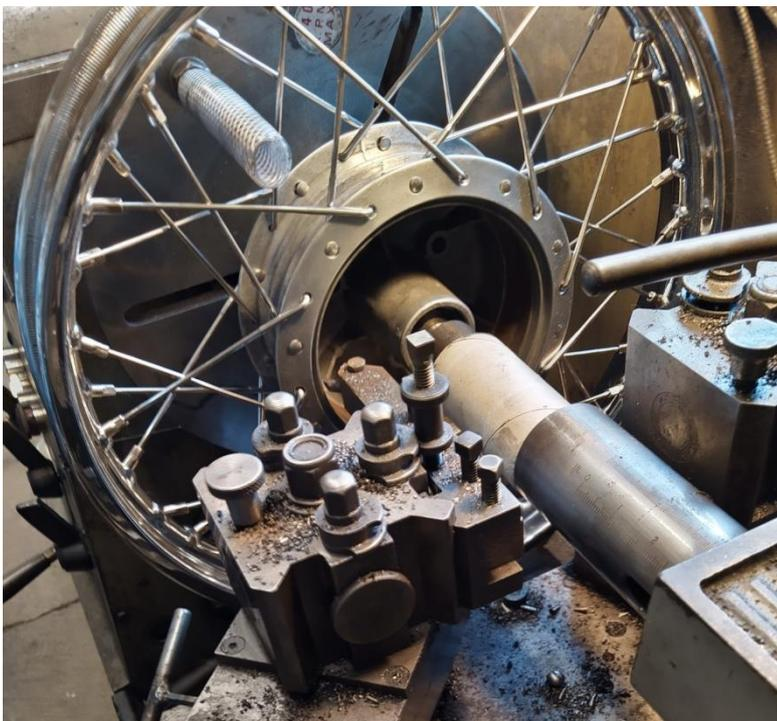
We regard brake drum skimming as only half the job. The second stage is to turn the brake linings to fit the drum. This saves waiting for the linings to "bed-in" and greatly reduces the tedious business of setting up a twin leading shoe brake. With the Velo 7 1/2 " front brake, which has a large lining area, full bedding-in can otherwise take a considerable mileage.
