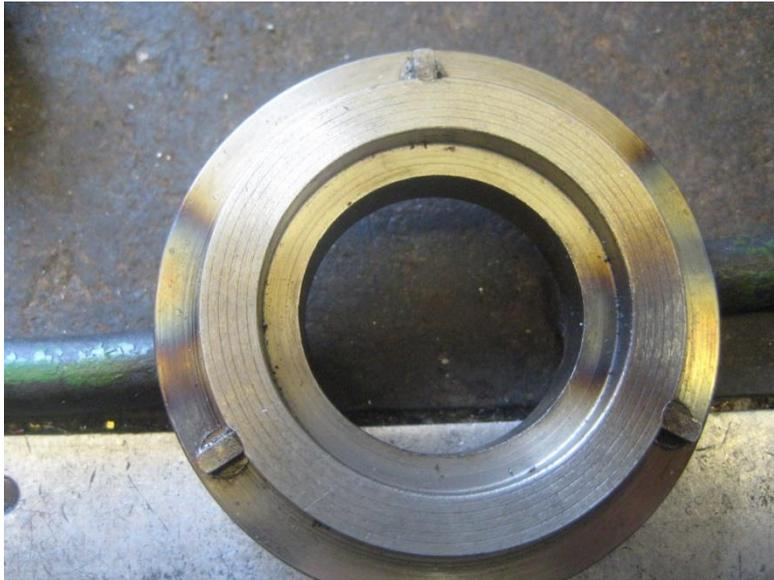
This picture shows our version of the Veloce tool, rather than locate from the bore of the bearing as the Veloce tool does, ours locates from the bore of the lock ring. It is also advisable to use a bolt and large diameter washers to hold the tool in place while tightening the ring.
