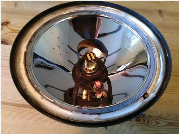
Wipac 7inch unit secured inside the original 8inch unit
