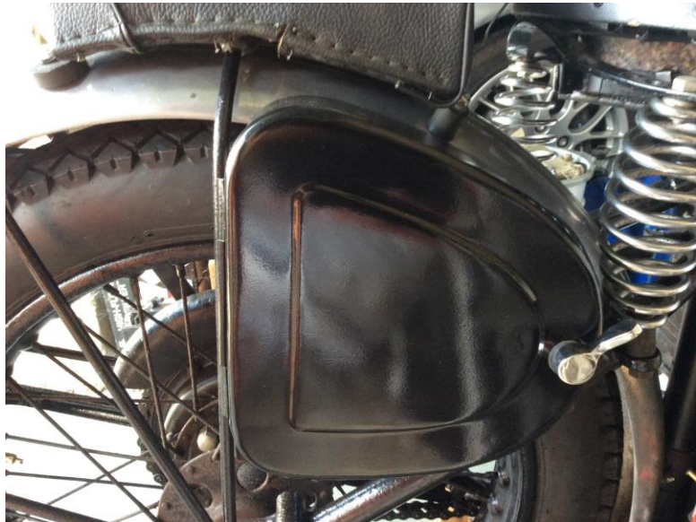
New tool box in place
