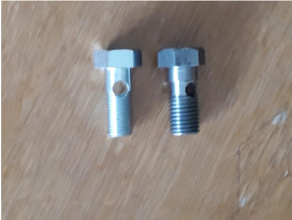
M 214 banjo bolt left, oversized 7/16 BSF banjo bolt right
